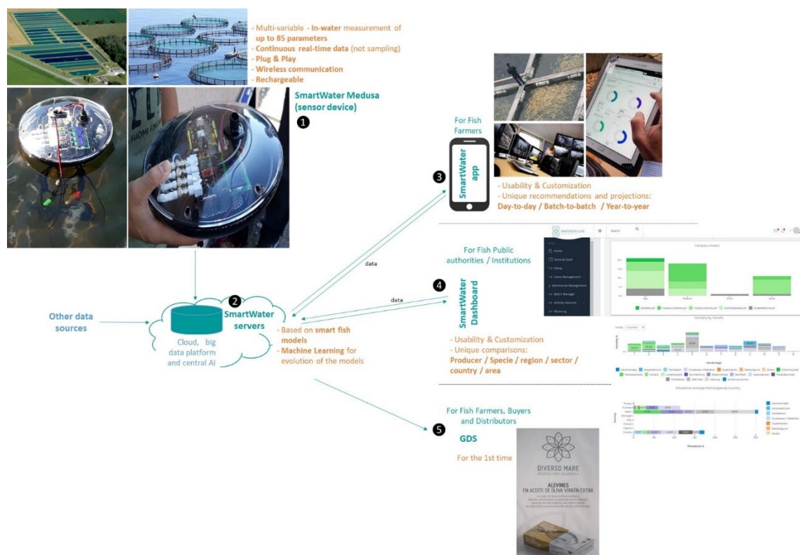
Figure 1: Medusa water quality parameters data collection architecture.
